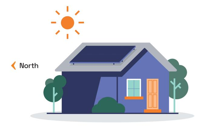
When designing your home, you will need to consider the roof orientation, pitch and available space for the Solar PV system so it is able to receive solar radiation and generate electricity. When your Solar PV system faces the street, you will need to consider the visual impact on the streetscape and could install the system flush on the roof. Doing this will also save you money by avoiding additional costs of mounting systems.
