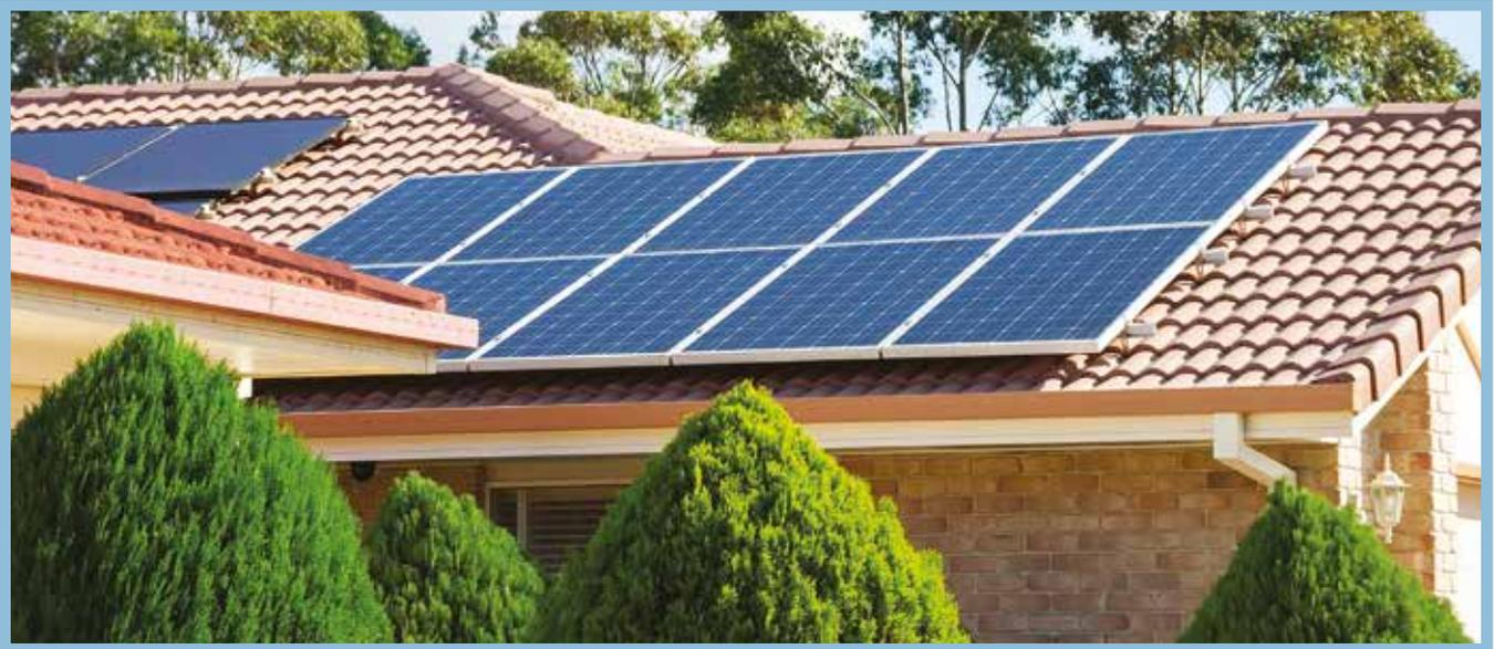
Before installing a solar PV system, you'll need to ensure the panels will be in a sunny area. They should also slope at an appropriate angle and face the right direction. Solar panels work best if installed facing north at 30 degrees from horizontal. If you install the panels with the wrong slope or direction it will reduce the amount of power generated.
