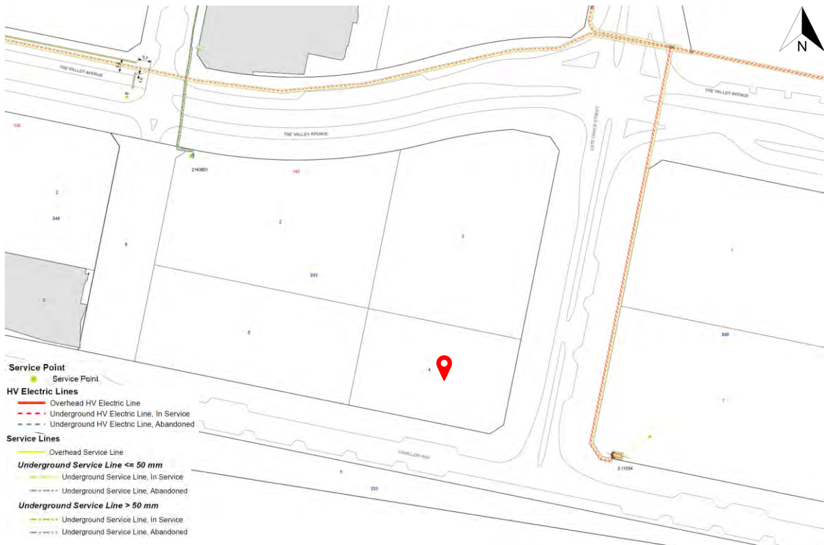
Figure 47 – Electrical BYDA Information (Evoenergy, 2024)
